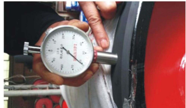
Hardness Test of Pulley Lagging
