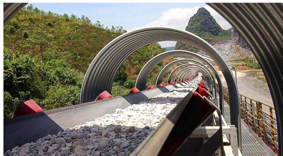
Mining Belt Conveyor
