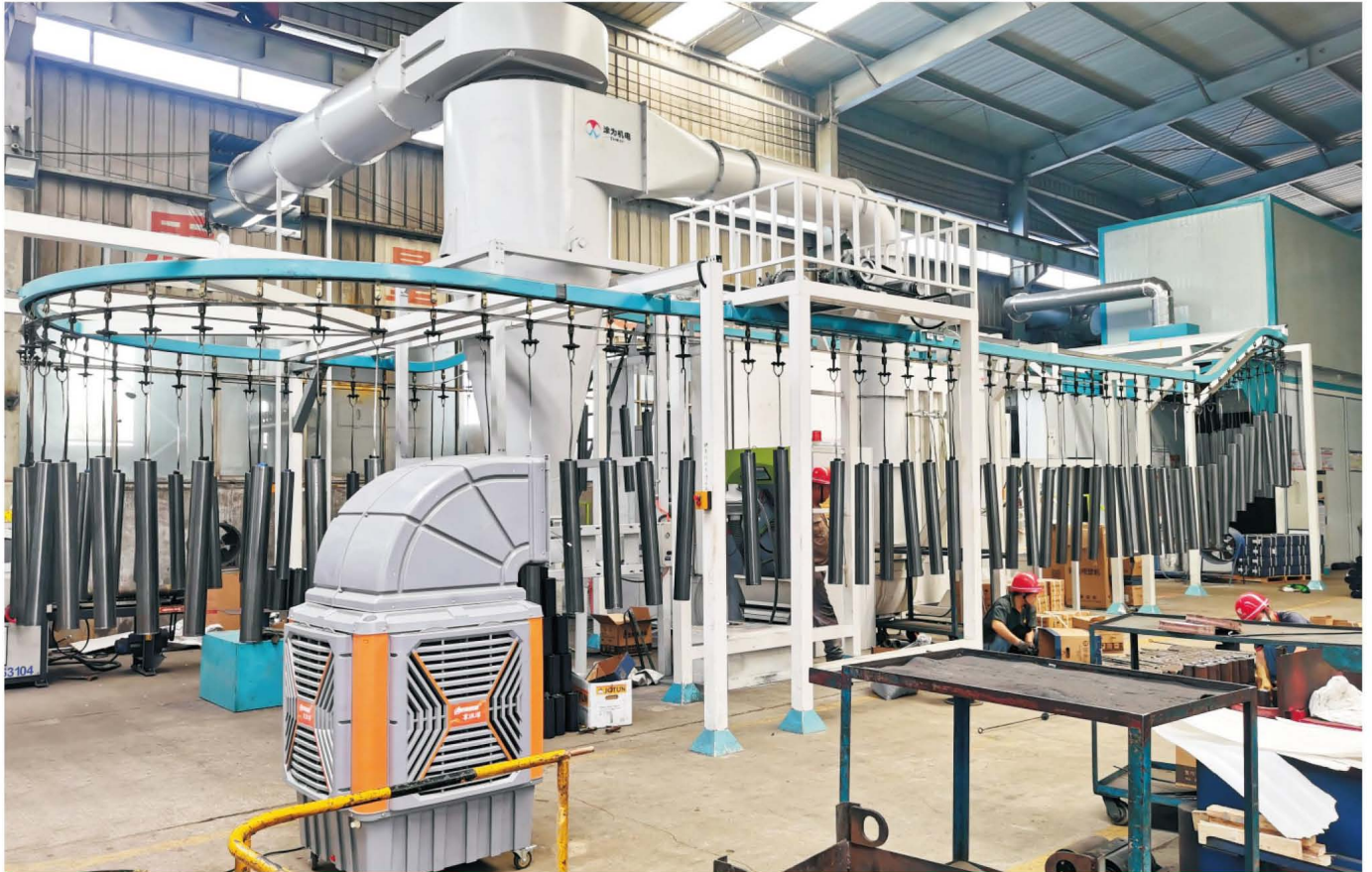
Automatic Spray Production Line
