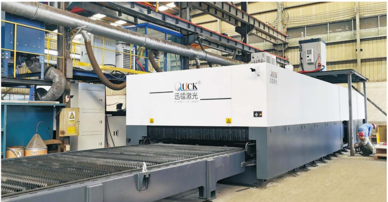
Laser Cutting Machine (20000W)
