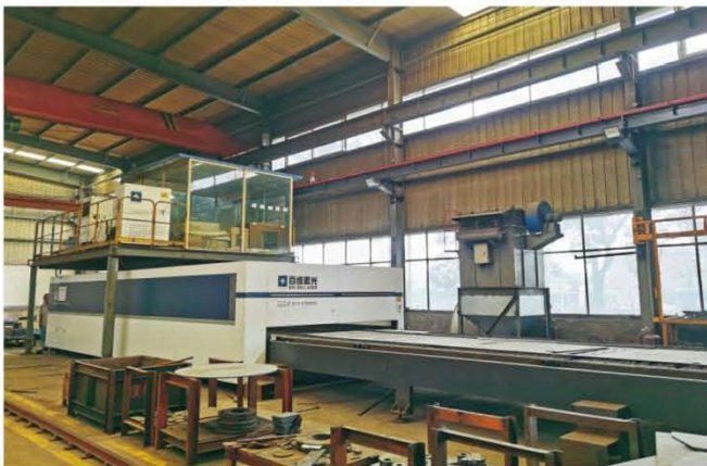
Laser Cutting Machine (6000W)
