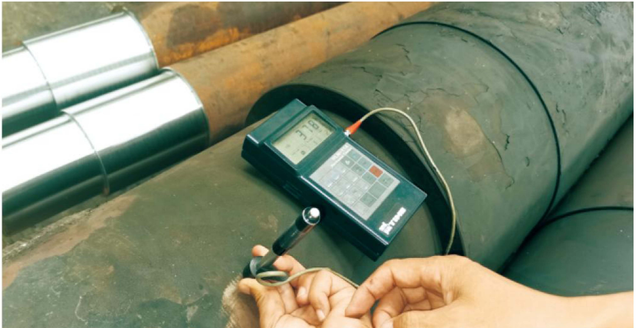
Hardness Test of pulley shaft After Heat Treatment
