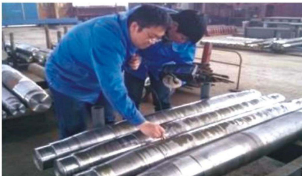
Ultrasonic Testing of Pulley Shaft
